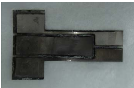
Fig. 2 IPMC with selectively grown multiple electrodes
