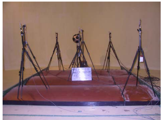
Fig. 8 Installation of laminated reflector for the measurement of random incidence sound absorption
