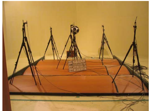
Fig. 7 Installation of acoustic reflector for the measurement of random incidence sound absorption
