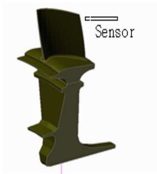
Fig. 4 Shape of bladed disk. a optical point sensor is located near the trailing edge to measure circumferential tip deflection.
