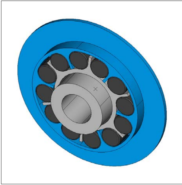
Fig. 1 FEM model for elastic coupling with rubber type circular segments
