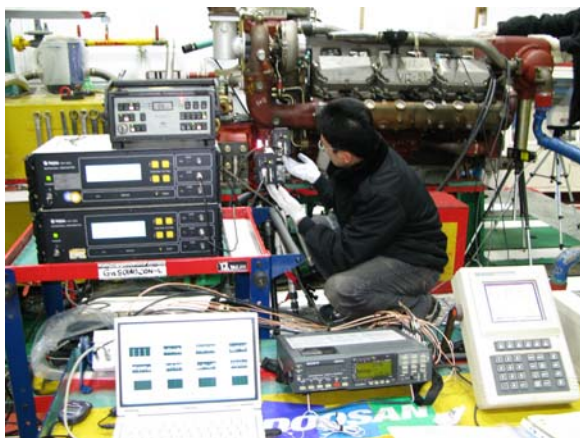
Fig. 10 Laser torsion meters for torsional vibration and adoption test of elastic coupling
