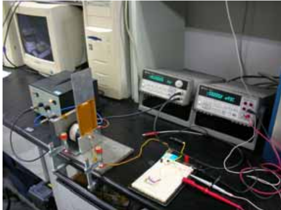
Fig. 5. Experimental Setup for Piezoelectric Energy Harvesting System
