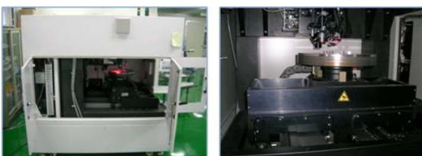
Fig. 1. Image of sapphire wafer drilling system
