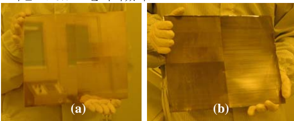
Fig. 4 Photograph of (a) Master pattern (b) Replicated nickel stamp
