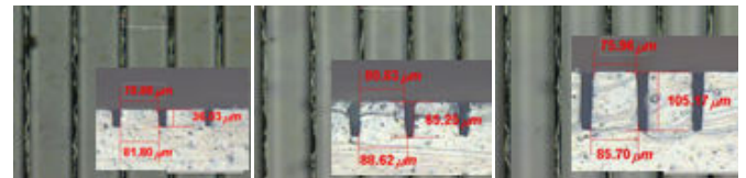
(a) pattern A (b) pattern B (c) pattern C Fig. 7 Machined micro channel structures and surface conditions
