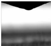
Fig. 6 Initial meniscus after leaving the nozzle for 30 minutes.
