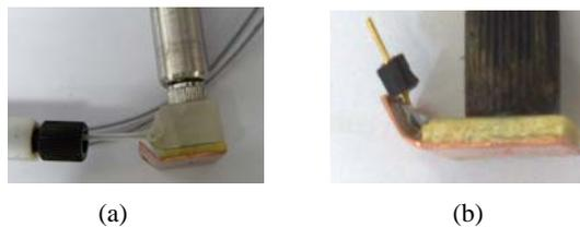
Fig. 5 Holding and ink flow mechanism and connection of the power supply to nozzle
