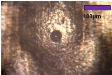
Fig. 4 Fabricated nozzle orifice through EDM
