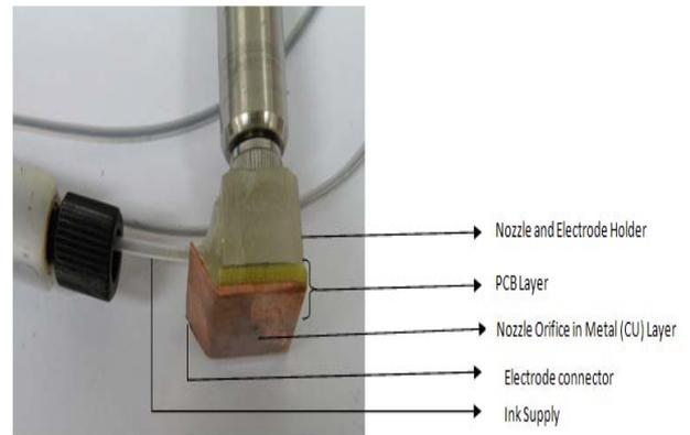
Fig. 1 PCB based Nozzle Head
