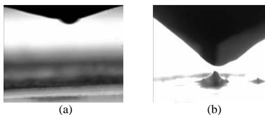
Fig. 7 show the response of the nozzle after applying the potential on the nozzle head. Figure (a) shows the initial response of the meniscus after applying the voltage and figure (b) shows the response of the nozzle after time t.
