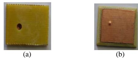
Fig. 2 Drilling of hole in the PCB nozzle (a) showing the top view through insulator (b) showing image through metallic layer (bottom side of PCB nozzle for the orifice design)
