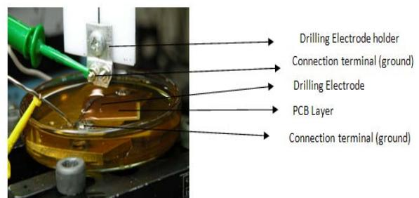
Fig. 3 EDM work on CU layer
