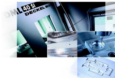
Fig. 2 Laser ablation and endmilling of mold (Deckel Maho)
