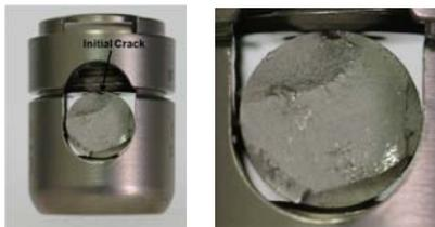
Fig. 3 Fatigue failure of spine fixation system with sand blasted surface
