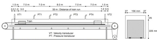
Fig.1. Schematic diagram of experimental layout [1]
