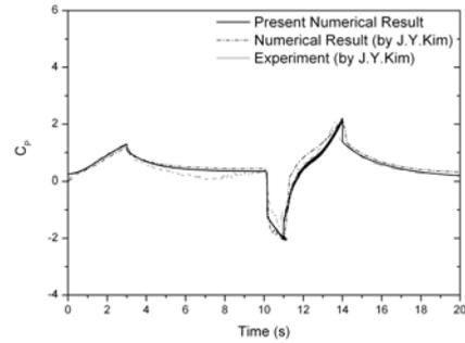
Fig.6 Comparison of  $C_p$  variations between experimental and numerical results at position of PT4.
