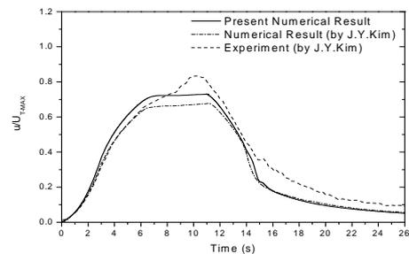
Fig. 8 Comparison of  $u/U_{T\_MAX}$  variations between experimental and numerical results at position of VT2.
