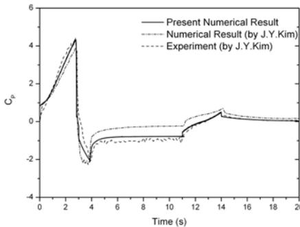
Fig.3 Comparison of  $C_p$  variations between experimental and numerical results at position of PT1.
