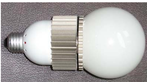
Fig.5 Prototype of proposed LED bulb
