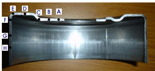
Fig. 4 Result of Hub preform for test deep-drawing
