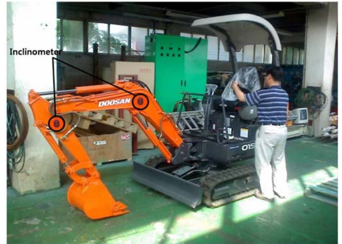
Fig. 3 Hydraulic excavator (SOLAR015) equipped with PVC and mounted inclinometer sensors
