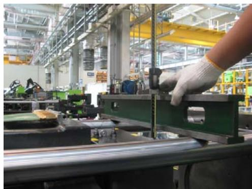
Fig. 3 Test block parallelism & concentricity set-up
