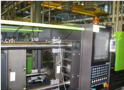
Fig. 5 Tie bar elongation test equipment set-up
