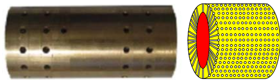
Fig. 5 Comparison between an orifice type and a metal foam
