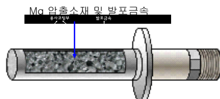
Fig. 6 Weight reduction using extruded Mg Material or metal foam
