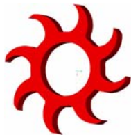
Fig. 2 Blade shape of an air turbine drive
