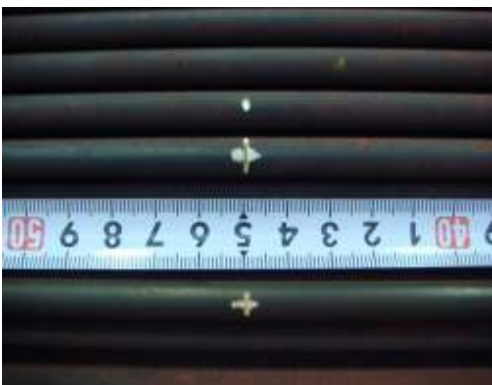
(b) Artificial crack
