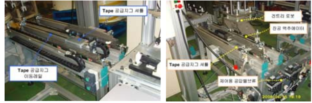
Fig. 7 Figure of taping system for sticking seal on door garnish
