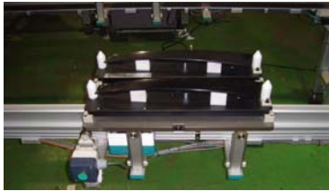
Fig. 5 Figure of wide-use jig for assembly door garnish
