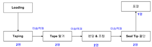
Fig. 2 Block diagram of current process for seal assembly
