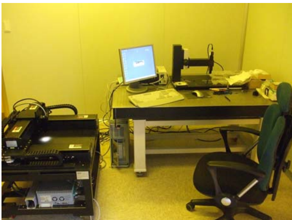
Fig.1 Optical measurement system on gantry-stage
