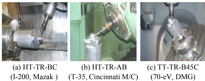
Fig. 3 5-axis machining and machined parts
