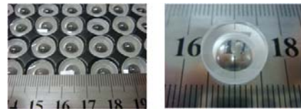
Fig. 8 Manufacture completed Glass Meniscus Lens
