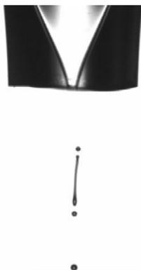
Fig. 1 Satellite droplets formed with isopropyl alcohol
