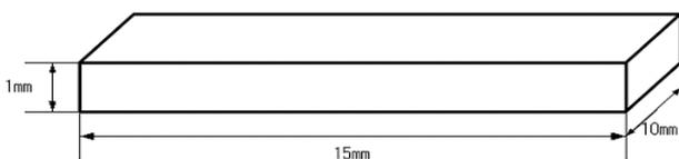
Fig. 1 Schematic diagram of the specimen
