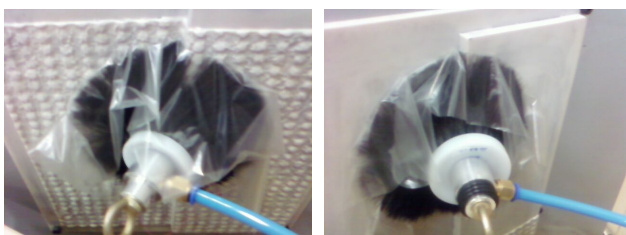
Fig. 2 Prototype of the vacuum attachment device
