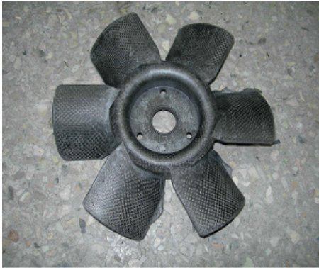
Fig. 6 Manufactured cooling fan using carbon prepreg
