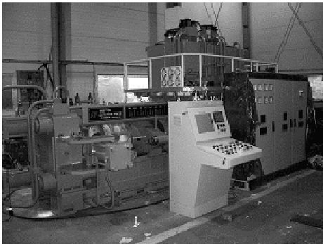
Fig. 3 Apparatus of CNC extruder with varied section
