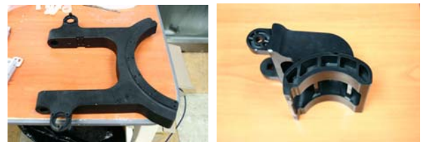
Fig. 3 Rapid prototype of a tilt arm and a gripper
