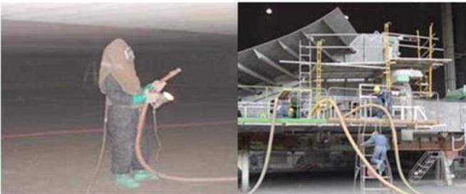
Fig. 2 Manual Blasting in the Double Hull
