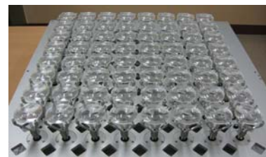
Fig. 8 8×8 Sun Collector with Sun Tracker
