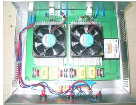
Fig. 6 Photocopy of the fabricated amplifier for driving two piezoelectric actuators
