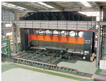
Fig. 1 Thick pipe forming using brake bending press
