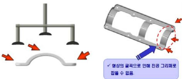
Fig. 1 Defect of vacuum gripping system
