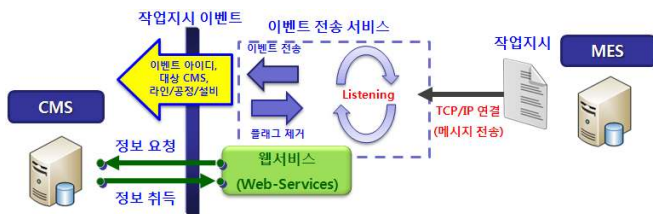
Fig. 4 Interface module for ERP/MES
