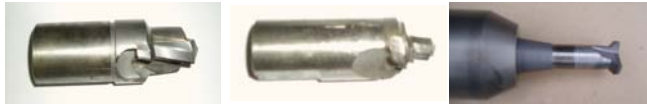
(a) P.C.D Drill (b) Air Hole Tool (c) P.C.D Back Counter Tool
