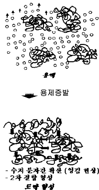
Fig. 6 Mechanism of coating film formation
