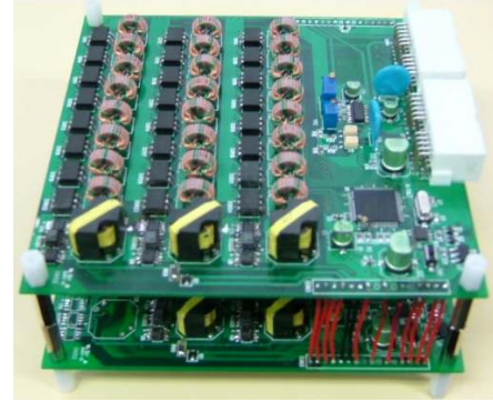
Fig. 3. Implemented engineering sample for 40 cells
