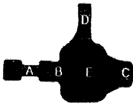
Fig. 1 Specimen positions in the thixoformed knuckle
