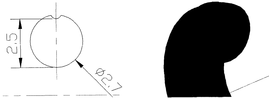
Fig. 5 The cross-section and dimensions of key home O-ring
