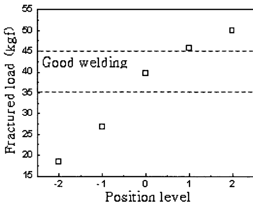
Fig. 3 Relation between stopper position and Fractured load
