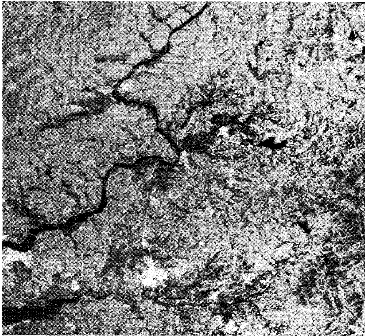
Figure 5. The RGB color composites are a combination of coherence images (R: 9807-9808, G: 9802-9804, B: 9802-9807)
