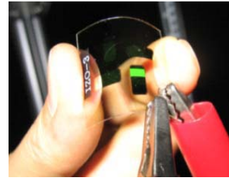
Fig 3. Green phosphorescent OLED using a-IZO
