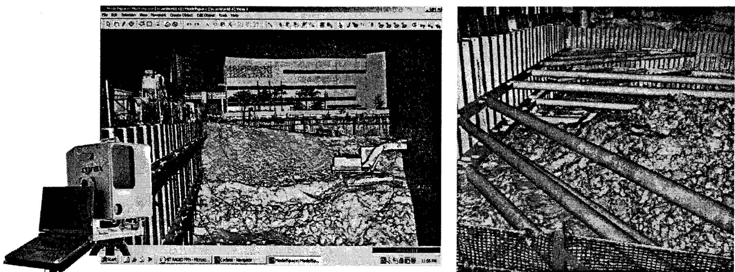
Figure 3. 3D Laser Scanning for Constructing 3D As-built Data
