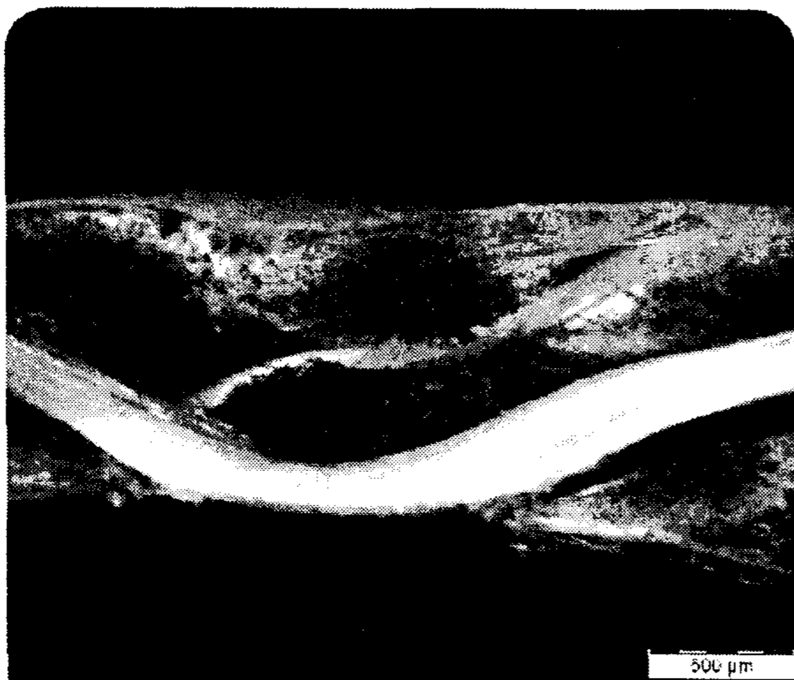
Fig 2. Cross-section of GORE™ membrane laminated to woven fibreglass fabric
