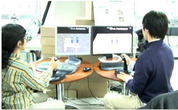
Figure 8: The test-bed system for collaboration over LAN where users each has a joystick and the two displays are identical
