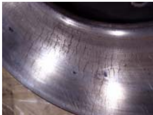
Fig. 1 Thermal fatigue cracks on disk surface
