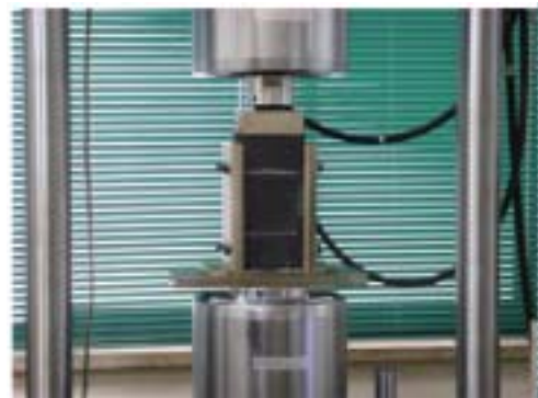
Fig. 6 Compressive test of the repaired specimen.
