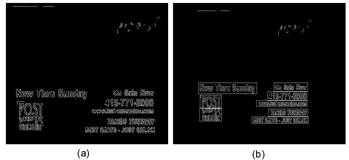
Figure 4. Coarse to fine projection. (a) Edge image after multi-frame integration. (b) Text detected regions.
