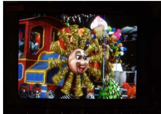
Fig. 3. Captured image of a 15-inch diagonal CNT-FED with double-gate structure.
