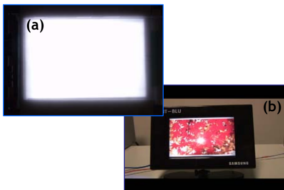
Fig. 5. (a) A Light image captured from 7-inch diagonal CNT-BLU with diffuser sheet: the gap between diffuser and BLU is maintained at 5 mm. (b) LCD picture image backlit by (a).
