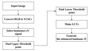
Fig. 1. The flow chart of adaptive contrast stretching
