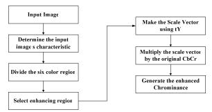
Fig. 3. The flow chart of adaptive saturation enhancement Method
